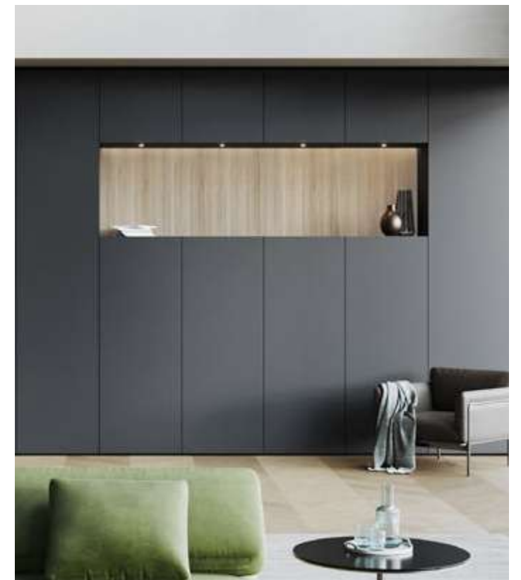
Recess panels in wood vertical or up to a height of one metre with horizontal veneer course possible. Vertical recess panels are butted in element widths.
